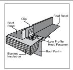
Fixed Clips are primarily used with these panels. Low profile head fasteners should be used with these panels to provide clearance for the panel over the fastener heads. These clips are manufactured from steel, stainless steel and other materials with various finishes to fit the needs of the panel application.
