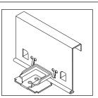
**Engineered panel clips**For standing seam panel attachments
