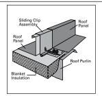
Fixed and Float Clips are used with these panels. The clips may have pre-applied sealant to maintain the panel seal at the clip attachment point. These clips are manufactured from steel, stainless steel and other materials with various finishes to fit the needs of the panel application.
